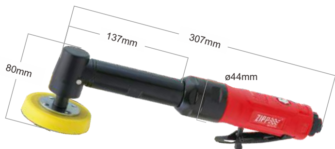
ZAP-342L 0.5HP (2,600RPM) Right Angle Buffer, 3" Diameter (3" Rotary Right Angle Polisher)
